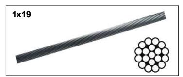
• 1x19 – Constructed of 19 individual wires which are twisted into a single strand. This design yields a semi-rigid product with minimal stretch. Generally, 1x19 cable can be used for most railing applications as it works well for straight runs or slight bends (up to 45°).
